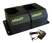
Dimensions: 181 x 102 x 57 mm Weight: 0,900 Kg Marking: CE / E-Mark Feeding source: AC: 100/240V 50/60 Hz Ingress protection: IP54 Charging status: red LED: charging / green LED: charged
